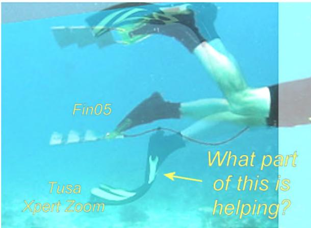
Preliminary testing has shown earlier versions of this to be more air-efficient than the best available split fins (the current standard). Air efficiency is an indicator of the overall effort required to move underwater.
