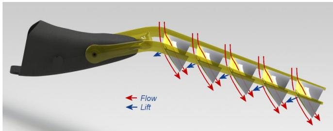
The vanes allow laminar hydrodynamic flow creating real lift and reducing drag. Other fins simply try to push the water out of the way creating turbulence and drag.
