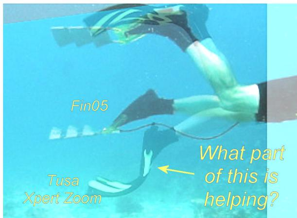
Testing has shown the Tusa Xpert Zoom to be nearest in air efficiency as the **MaxAir™** but it re-quires fast kicks to move effectively. This is very much like riding a bicycle. In first gear it is easy but it is difficult to go fast for very long. The hydrodynamically aligned vanes in the **MaxAir™** make swimming like riding a bike with an automatic transmission. With vanes always aligned at the proper angle of attack the
